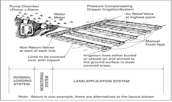
Figure 2: Schematic of a Subsurface Pressure Compensating Dripper Land Irrigation System. Source: Auckland Regional Council TP58 (2004).
