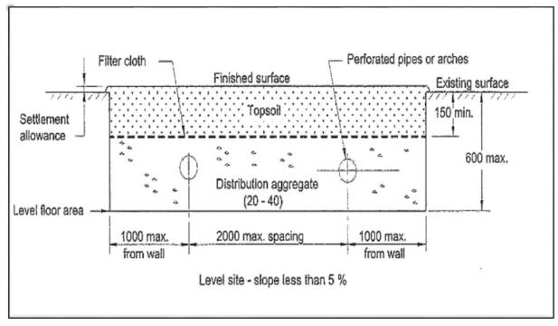
Figure 5: Conventional Bed Disposal Field System.
