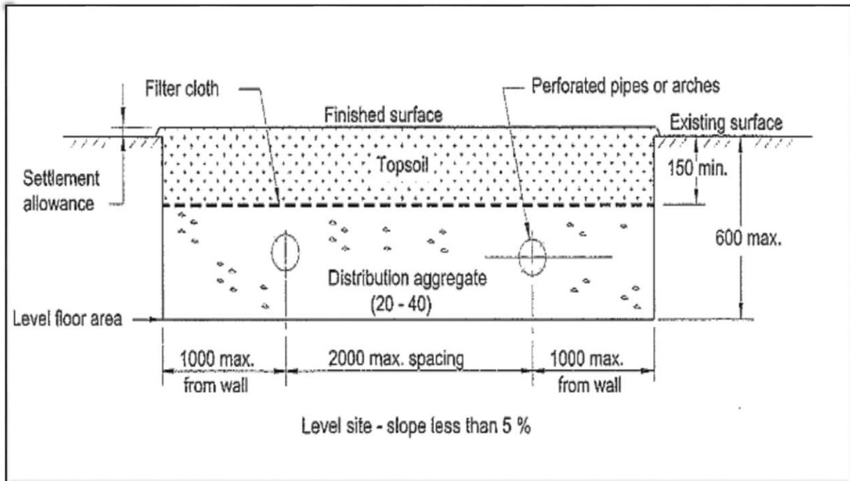
Figure 5: Conventional Bed Disposal Field System.
