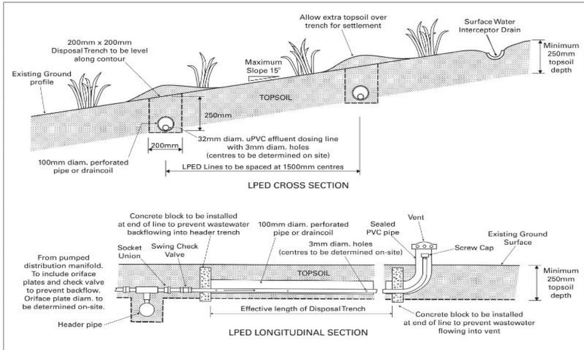
Figure 3: Example of a Shallow LPED Application System. Source: Auckland Regional Council TP58 (2004).
