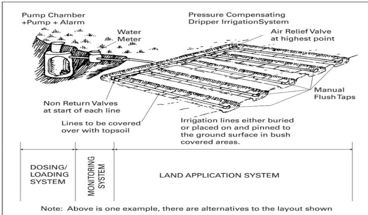
Figure 2: Schematic of a Subsurface Pressure Compensating Dripper Land Irrigation System. Source: Auckland Regional Council TP58 (2004).
